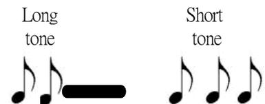
When intend to choose one of above options, simply position the throttle stick from minimum to maximum after the indication tone. The next step is to position the throttle stick back to the minimum position to confirm. You could now simply shut down the power. The selection was stored into the microprocessor when the throttle stick was in confirmation position.
