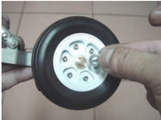
Step 9 (washer 10 x 0.35~1.0 mm) Add another washer on the axle.
