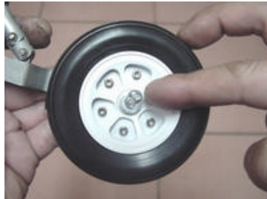
Step 10 (E Clip E-3.2) Add an E clip onto the groove in the axle.
