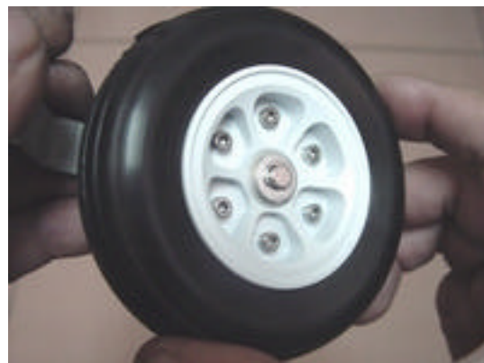
Step 12 Check the tire to make sure it spins smoothly. Check to see if there are any gaps between the wheel and E clip. In case there is a gap, add an extra washer as shown in step 9.
