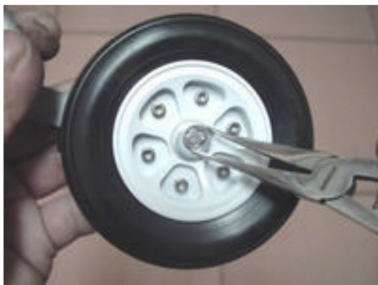
Step 11 Use a vice or similar tool to force the clip onto the axle groove.
