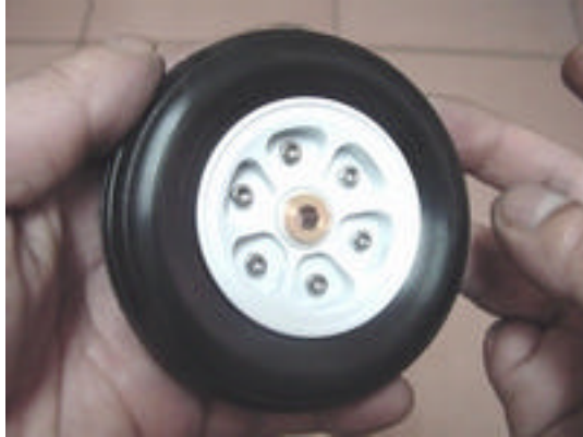
Step 7 Add some more lubricant to the bushing.
